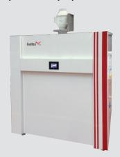
Climatic chambers for testing on products subjected to pressure or solvents (ATEX)
