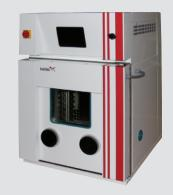
Chamber with viewing window and access holes with gloves for product handling
